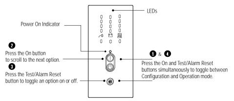
Figure 14. Using the Configuration Mode
